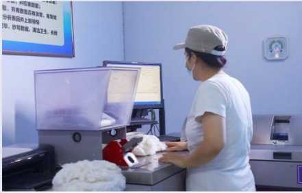
Uster HVI 1000: Large-capacity cotton analyzer: It mainly detects physical indicators such as raw cotton Micronaire, color, and strength, and other physical index.
