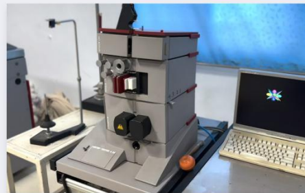
Uster Tester 4 SE: Evenness Tester: It mainly detects the changes of common yarn defects such as evenness CV, thick places, thin places, and neps in the yarn.
