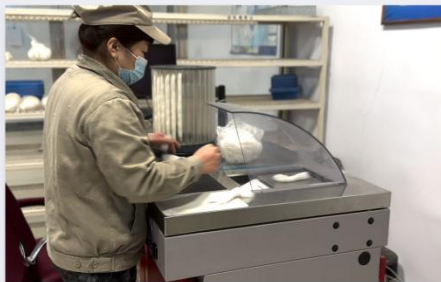
Uster AFIS PRO2: Cotton single fiber analyzer: It mainly detects the changes of fiber indicators such as fiber length, neps, short fibers, fineness and impurities during the process from cleaning to roving in the pre-spinning workshop, so as to optimize the production process and ensure stable quality.
